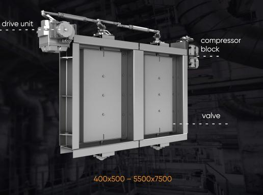
Pendulum valves are designed for the tight closing of dust silos that are operated under pressure different from atmospheric pressure and their discharge without decompression. The dampers are used within ash collecting and pulverization systems.
